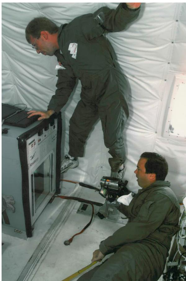
A 1999 low-gravity test of additive manufacturing aboard a KC-135 “Vomit Comet.” This early work was sponsored by NASA’s Marshall Space Flight Center. Image Credit: NASA
