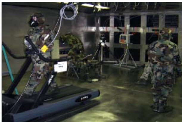
FIGURE 1 Man-in-Simulant Test exercises in the chamber. The PETMAN system is required to perform the same set of exercises as the soldiers shown. SOURCE: Charles Walker, U.S. Army Dugway Proving Ground.
