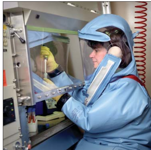
Work in a BSL-4 laboratory using a negatively pressurized laminar flow hood.
