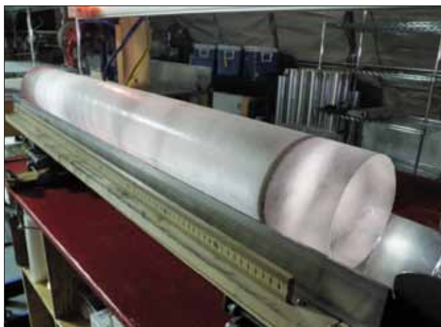
Figure 4. A one meter long section of ice core from the West Antarctic Ice Sheet Divide Ice Core. The visible dark layer shows deposits of ash. Measurements of air trapped in ice cores are used to create records of past temperatures and concentrations of atmospheric gases. Source: Heidi Roop
