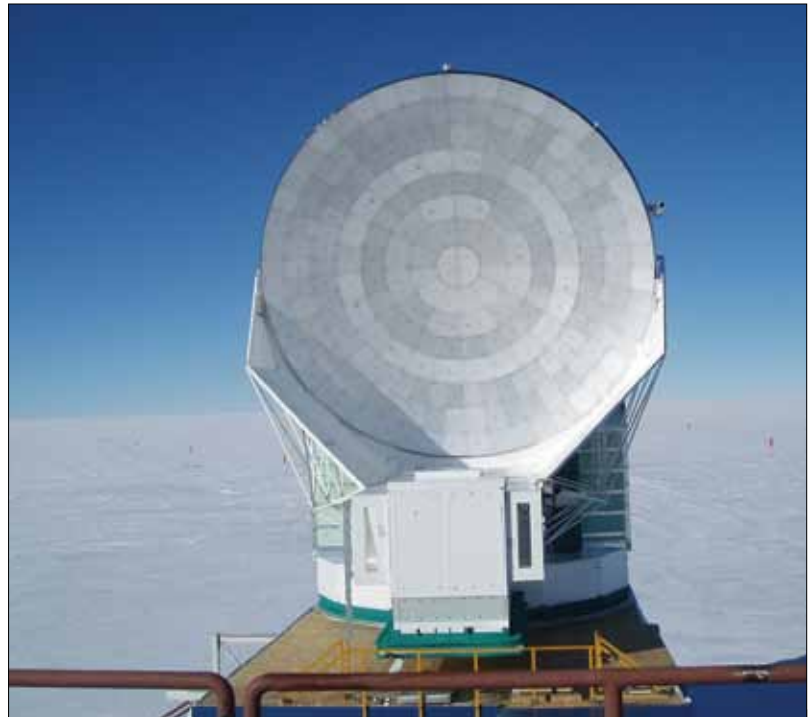
Figure 7: Telescopes can exploit the extraordinary transparent and stable atmosphere of Antarctica to map the intensity and polarization of cosmic microwave background radiation. Source: Edward Dunlea
