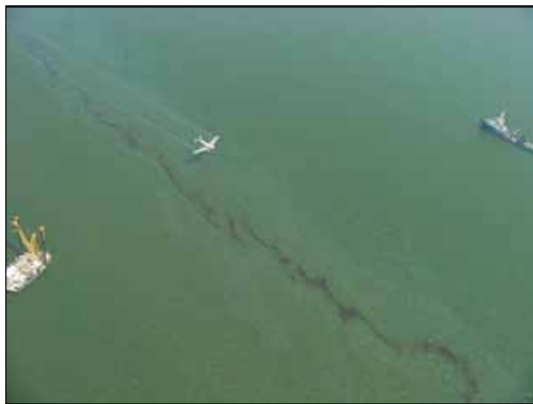
Figure 2. Dispersant is applied to an oil spill caused when the Tank/Barge DBL152 and the T/V Rebel impacted an obstruction off the Louisiana Coast in November 2005. Credit: NOAA Office of Response and Restoration.
