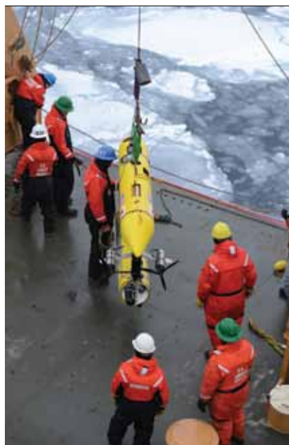
Figure 5. The crew of the Coast Guard Cutter Healy prepare to lower an unmanned underwater vehicle, operated by the Woods Hole Oceanographic Institution, into the Beaufort Sea during a simulated spilled oil response and recovery exercise. Credit: U.S. Coast Guard, Petty Officer 3rd Class Grant DeVuyst.
