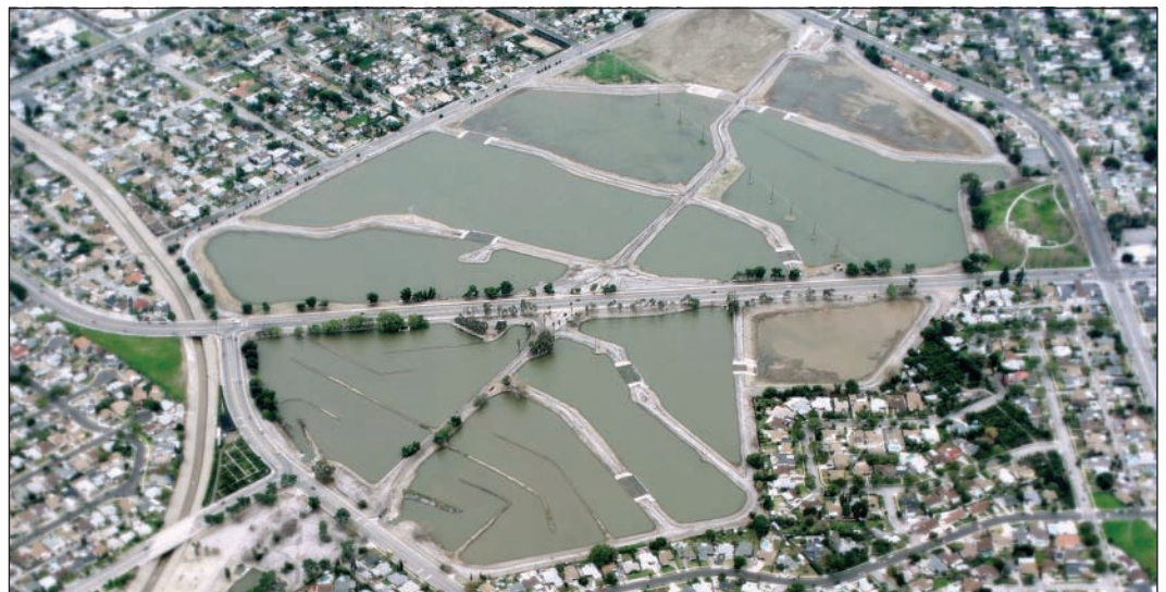
Figure 2. Several impoundments in California capture and store stormwater for groundwater recharge. The Rio Hondo Spreading Grounds, pictured here, receive controlled releases from the San Gabriel Canyon, Santa Fe, and Whittier Narrows dams. SOURCE: Department of Public Works, Los Angeles County.
