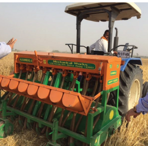
FIGURE 1-2. Wheat seeder designed to eliminate crop waste burning in rice paddies in India.
